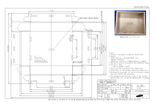
Fig. 2-2. Inner box package drawing.
